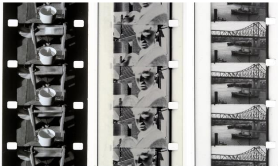
Reversal (camera original positive, solid black edge), Negative copy (clear edge), Print (clear edge or solid black edge depending on printing)
